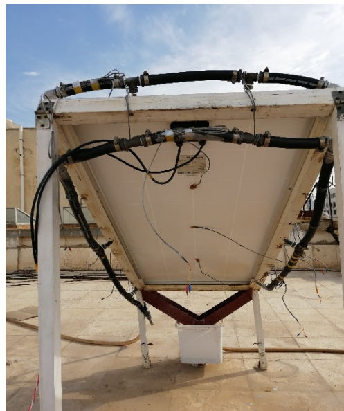
Figure 2. The front and backside of the PV panel with the specific water nozzle system.
